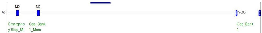
Figure 3: Capacitor Bank-1 Output Logic
