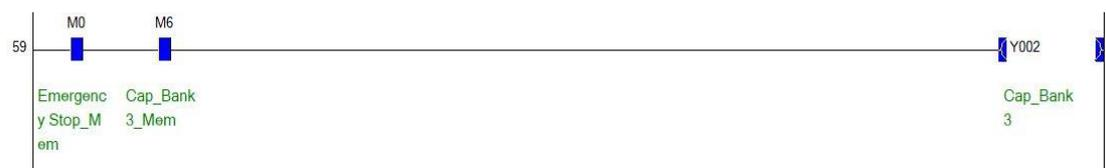
Figure 7: Capacitor Bank-3 Output Logic
