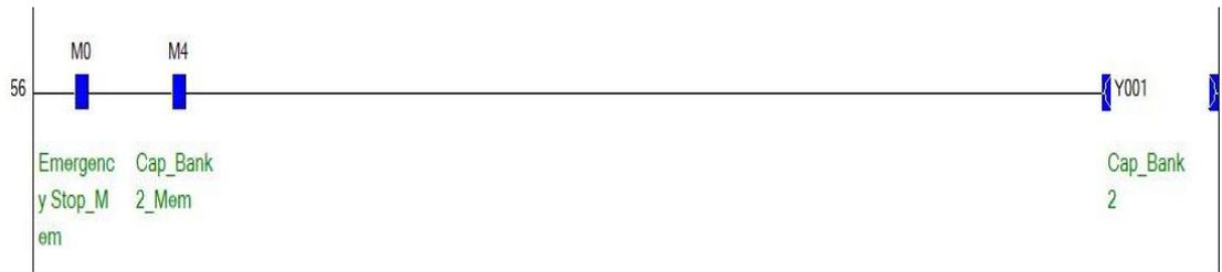
Figure 5: Capacitor Bank-2 Output Logic
