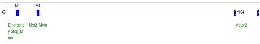
Figure 6: Motor-2 Output Logic
