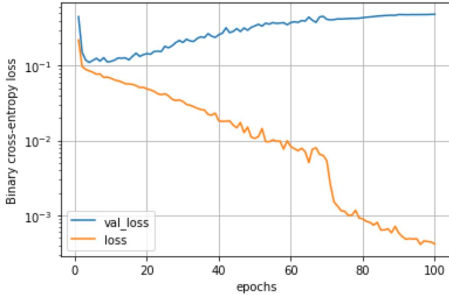
Figure 6: Binary Cross Entropy loss for Nakagami fading channel
