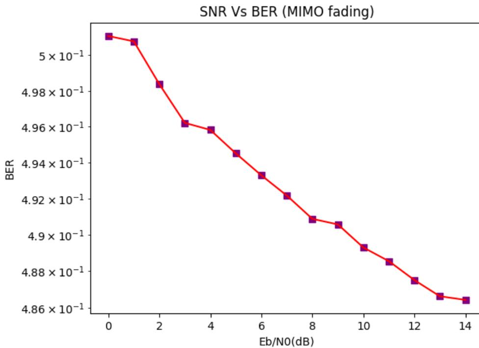
Figure 9: BER for MIMO fading
