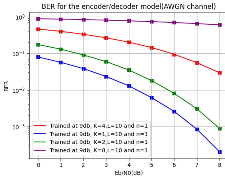
Figure 4: SNR vs BER for different k
