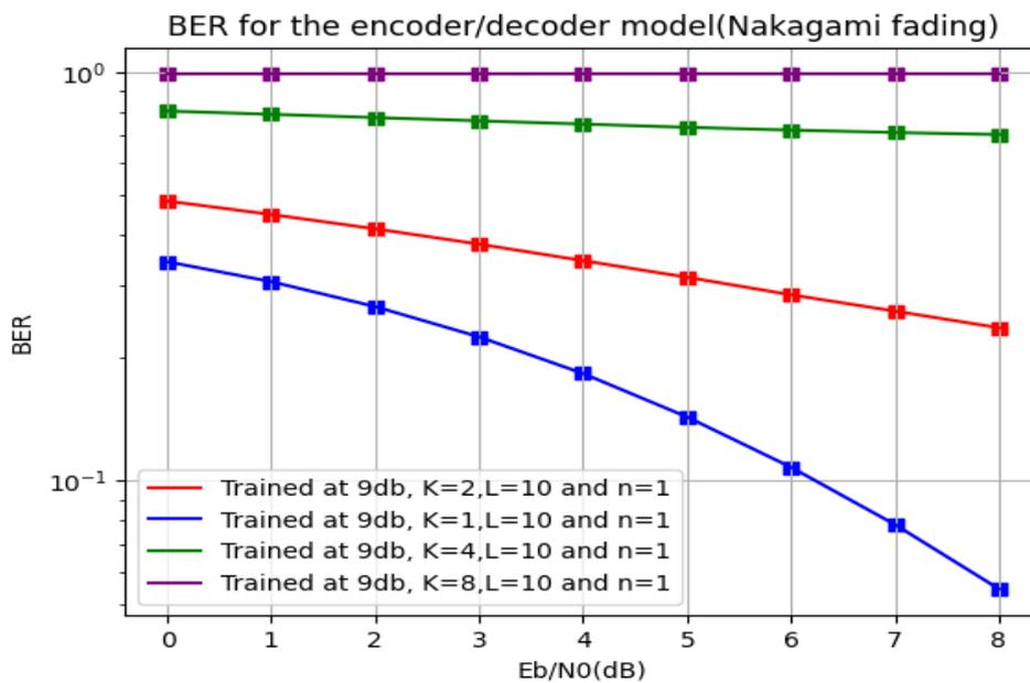
Figure 7: SNR Vs BER for different  $k$  under Nakagami fading
