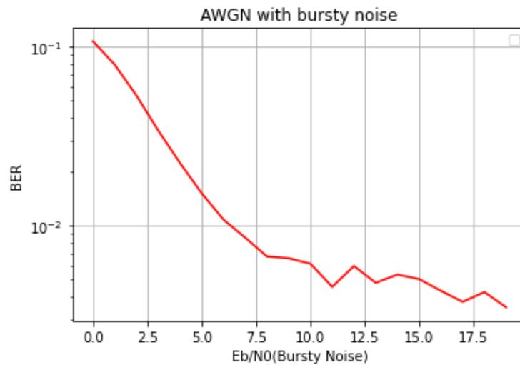
Figure 5: SNR vs BER for Bursty AWGN
